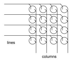
When a switch is closed, it establishes the connection between a line and a column
